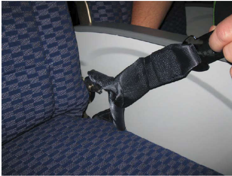
Figure 7 - Seat Y-belt misalignment
