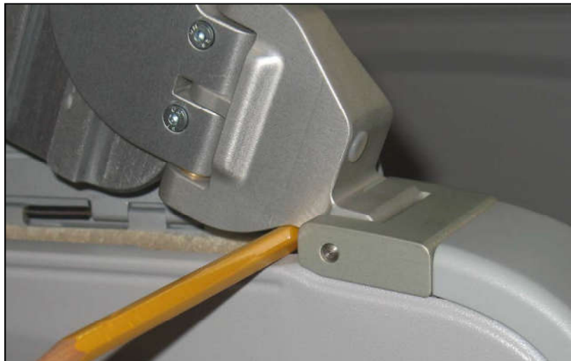
Figure 16 - This is a hinge for an in-arm tray table. It is an example of a type 1A score from the injury potential analysis table.
