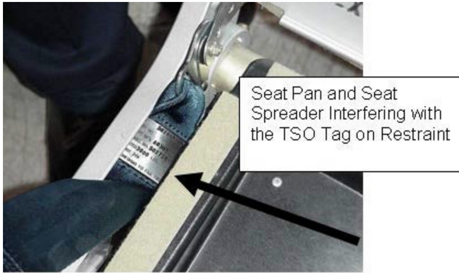
Figure 4 - An example of a design to avoid
