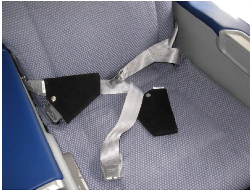
Figure 8 - Belt cover non-permanent attachment
