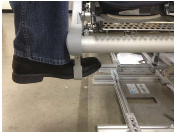
Figure 27 - Acceptable foot insertion into stirrup-type step
