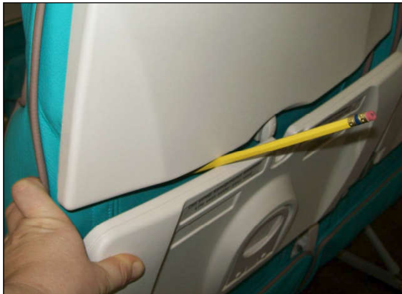
Figure 18 - This is an aft mounted food tray table. It is an example of a type 1A score from the injury potential analysis table.
