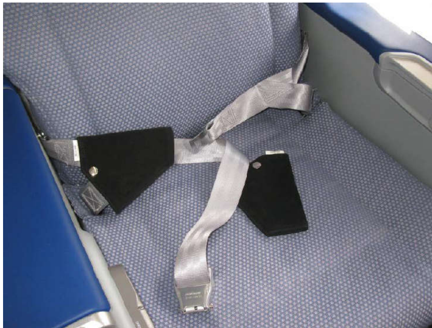
Figure 8 - Belt cover non-permanent attachment
