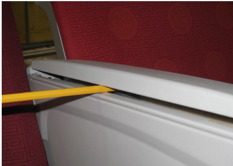
Figure 15 - This is the arm cap for an in-arm tray table seat. It is an example of a type 1a score from the injury potential analysis table.
