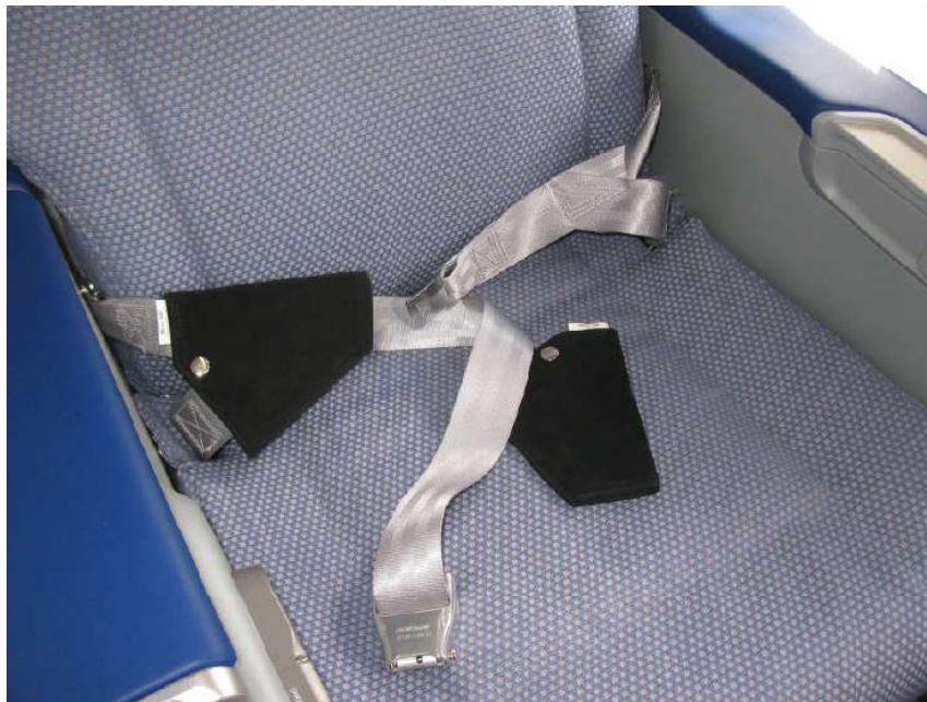
Figure 8 - Belt cover non-permanent attachment
