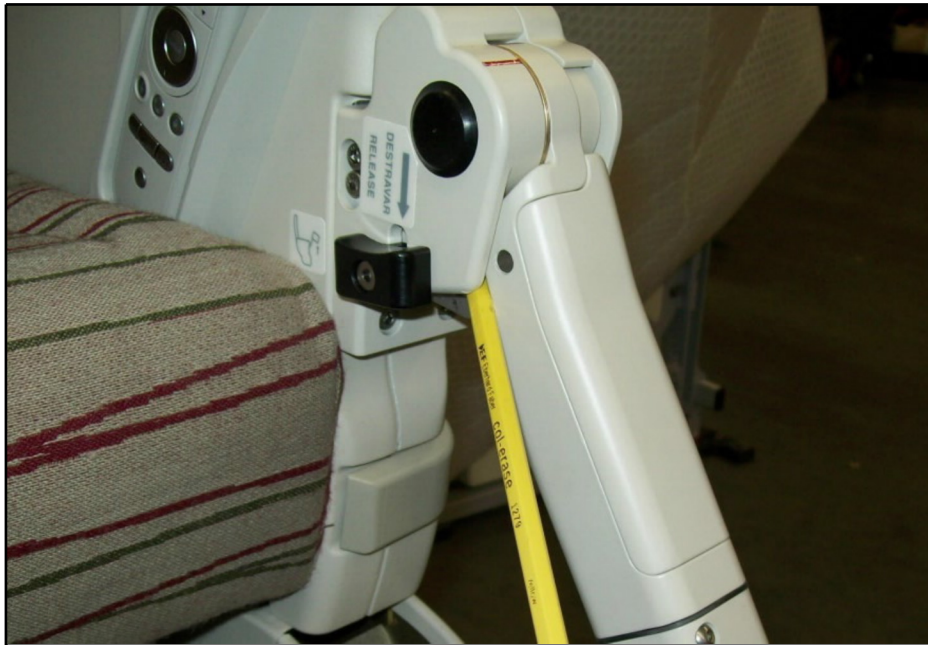
Figure 14 - This is the hinge for an in-arm video display. It is an example of a type 1a score from the injury potential analysis table.
