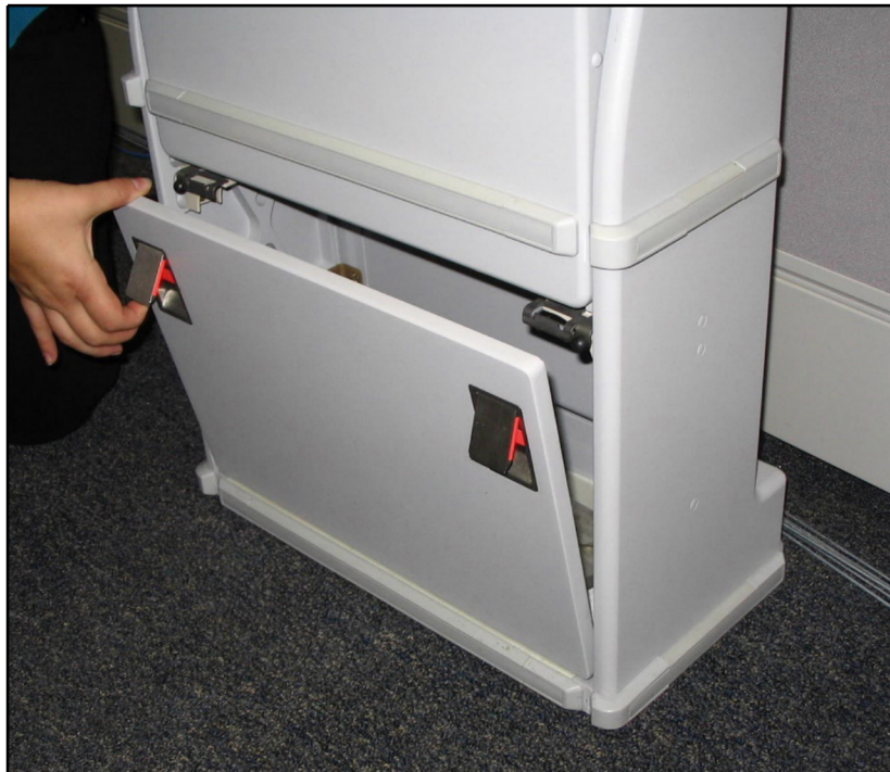
Figure 17 - This is a spring-mounted stowage box door. It is an example of a type 4a score from the injury potential analysis table based on spring force potential.
